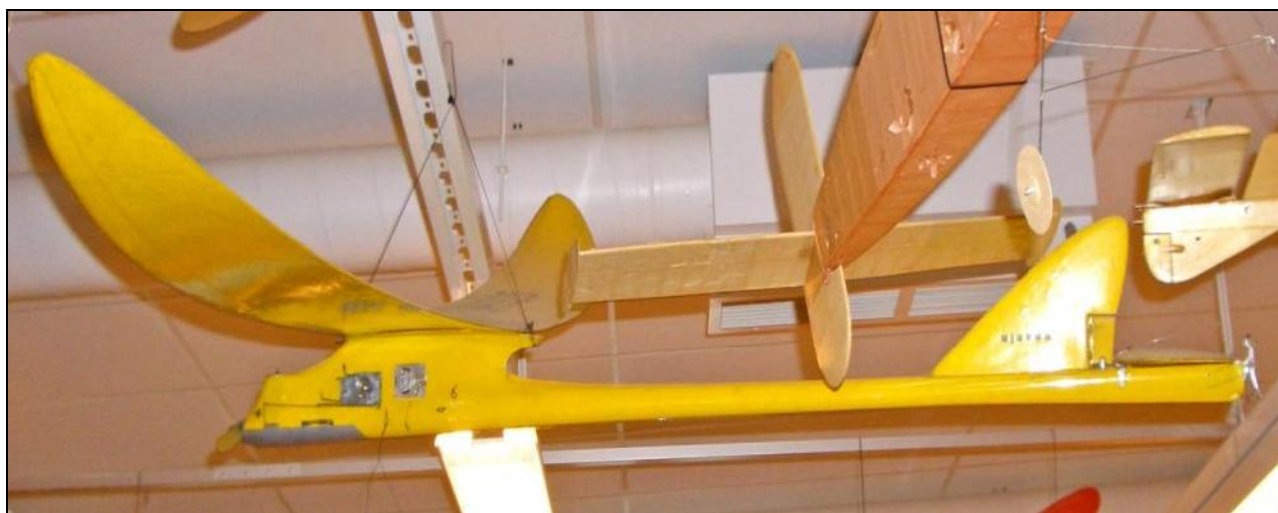
Ujakka, with elliptical dihedral, mechanical timers, VIT and AR !
