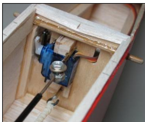
Right: Servo mount and pushrod linkage on rear-side of escapement former. Note also torque-rod linkage to escapement linkage on front side of former
