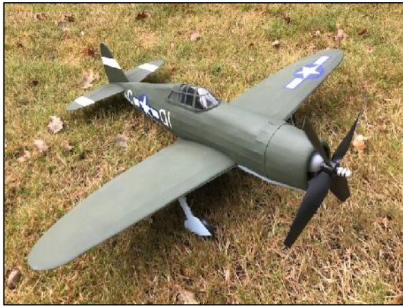
1.5x enlarged rubber-powered Thunderbolt from Flying Scale Models of WWII. Designed by E.I.Coleman.
