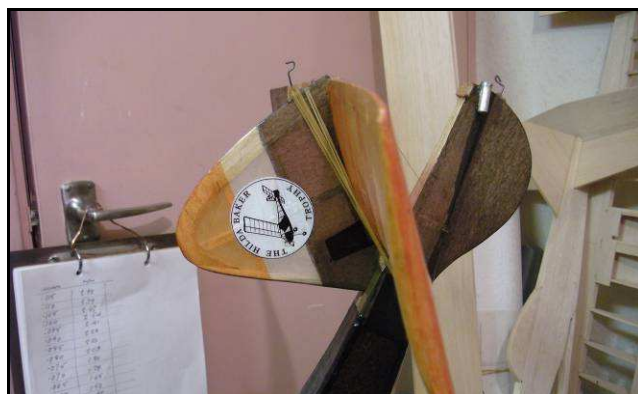
My ' Tomboy ' tailplane has locating dowels at the rear, and the front is located by the fin in a slot
