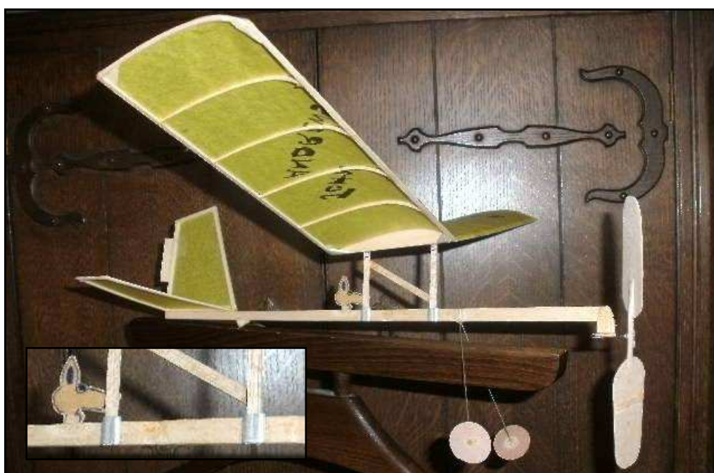
My Rat with the flattened aluminium tubes for the plug-in wing Mr Rat has had his nose put out of joint by the rearward repositioning of the wing
