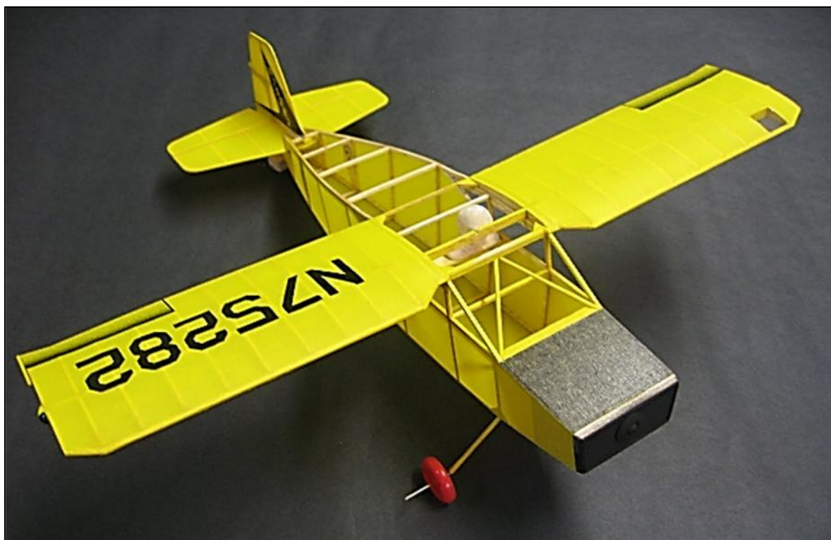
Fig 9 Nesmith Cougar Peanut in assembled state nearly ready for fitting top stringer and covering. The fin has not yet been glued into position and the wing is just resting. Must do something about those red wheels!
