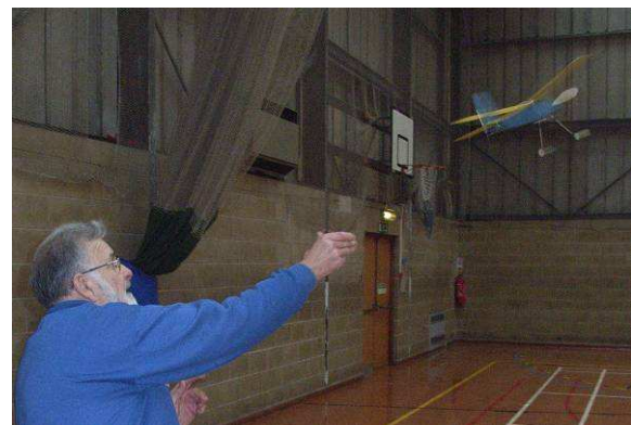
Just to show that these half-size Wakefields do fly we have Mike Brown, again, sending his 'Jaguar' and his '36 Copland' on their way. Just for the record these models are powered by a 15" loop of rubber with about 1000 turns driving an 8" diameter propeller.
