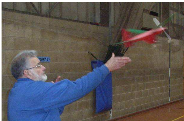
Just to show that these half-size Wakefields do fly we have Mike Brown, again, sending his 'Jaguar' and his '36 Copland' on their way. Just for the record these models are powered by a 15" loop of rubber with about 1000 turns driving an 8" diameter propeller.
