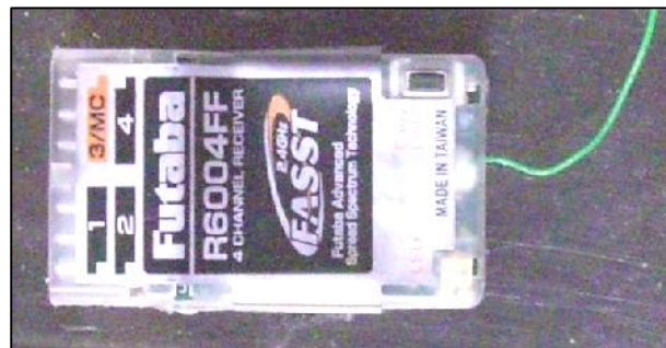
NOT suitable for F/F, typical "Indoor-type" R/C Rx have very limited operating range. JR weighs 2.0g Futaba weighs 3.3g. Note tell-tale single wire antenna and micro-JST style connectors.
