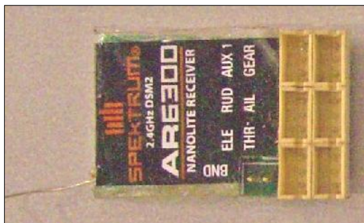
NOT suitable for F/F, typical "Indoor-type" R/C Rx have very limited operating range. JR weighs 2.0g Futaba weighs 3.3g. Note tell-tale single wire antenna and micro-JST style connectors.
