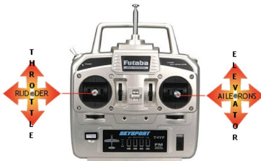
Typical R/C transmitter, set up for Mode 2 control, with Throttle on Left joystick
