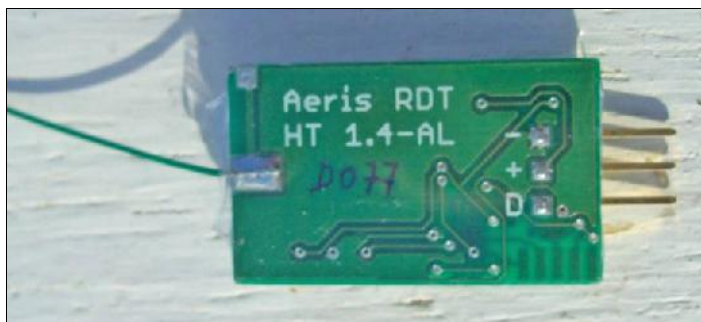
Aeris RDT Rx unit small and lightweight at only 2.5g
