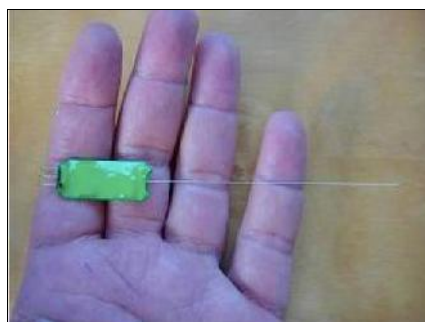
Ken Bauer's Airtek RDT Rx with 3 inch antenna, is smallest and lightest known full-range unit weighing just 1g
