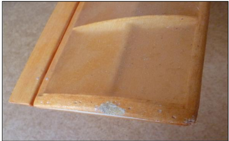
Rodent damage, they really like rubber. Look at teeth marks in T/P tip block.
