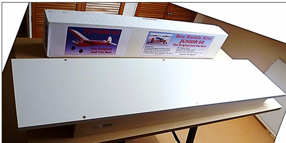
Treated myself to a new building board for 2017. 4' by 1' shelf board screwed to 2 two wooden batons. This will have cork tiles glued to it. It's totally flat, very strong, and doesn't warp.
