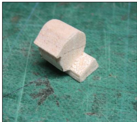
Fig 2. Sawn pilot profile with head sides cut away to form shoulders.
