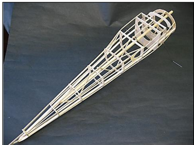
Fuselage frame before removal of the temporary structure. The final stringers need to be added.
