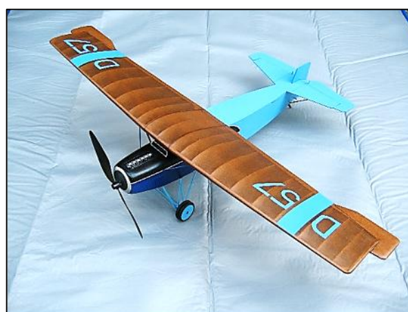
31.5" wingspan Peter Rake designed Fokker FII, weight 205g. It started out with a GWS 8x4.3 propeller, but I changed it to an APC 7x5 (left) for greater ground clearance. Mine's not resting on an elephant's trunk (see last month's NC)!
