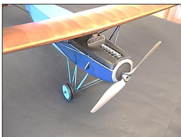
31.5" wingspan Peter Rake designed Fokker FII, weight 205g. It started out with a GWS 8x4.3 propeller, but I changed it to an APC 7x5 (left) for greater ground clearance. Mine's not resting on an elephant's trunk (see last month's NC)!
