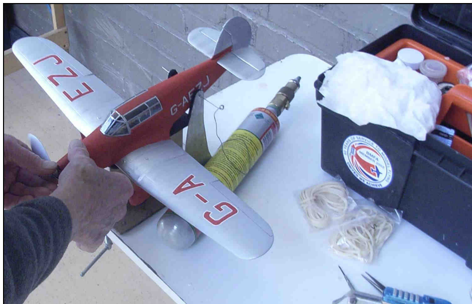
The 'Vega Gull' has the nose block inserted after winding.
