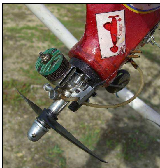
Front end of Phil's Champion with original K&B Greenhead .09 and Master 7 x 4 Prop which is allowed 20 second engine run.
