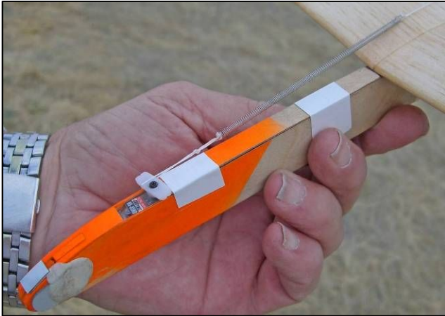
Todd Reynolds Tip Launched Glider simply hooks DT line directly over servo arm (Note, only viable for low line tension)
