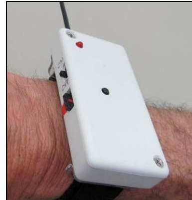
AirTec airborne RDT system: Rx; servo; and LiPo: Ken Bauer's wrist strap mounted AirTec RDT Tx
