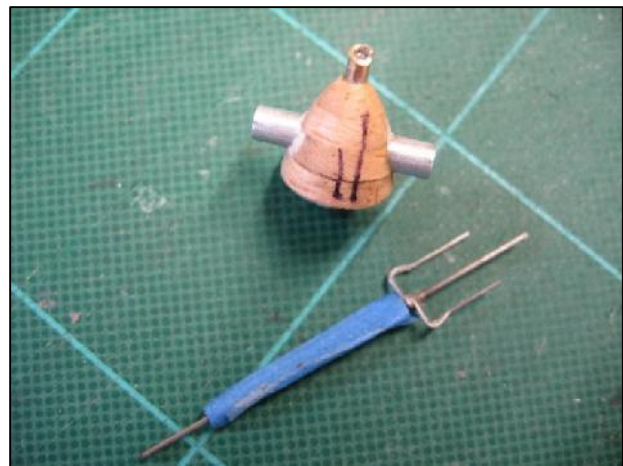
Fig 4. Balsa spinner with brass hub tube and aluminium cross tube for propeller blades, with wire trident used for forming the spinner
