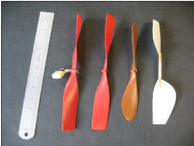
Fig 1. Red Slick Streak prop on hanger as supplied with the North Pacific ARTF, 5.5 in dia. Slick Streak prop, brown 4.75 in Peck prop, 5 in yoghurt carton prop
