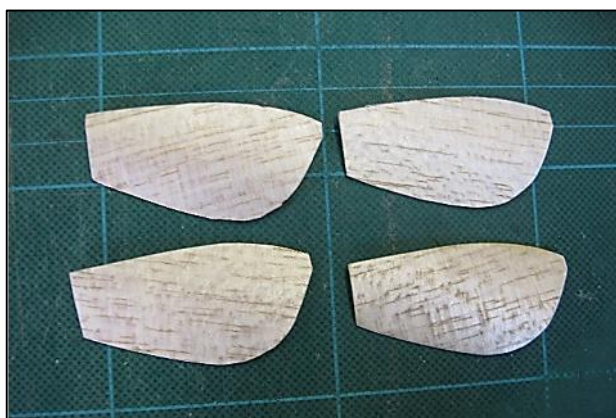
Fig 9. Formed balsa blade laminae. Note grain direction.
