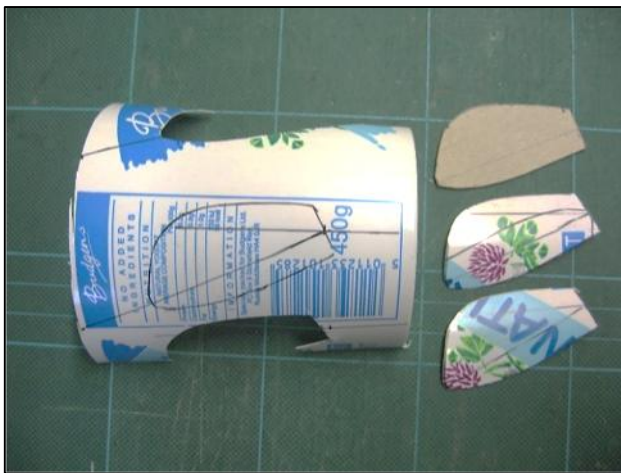
Fig 5. Marking out and cutting blades from large yoghurt pot using card template
