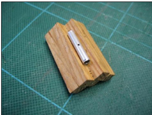
Fig 3. Wooden vee-block to aid drilling of hole in 5/32 aluminium tube.
