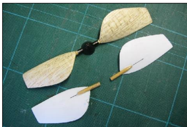
Fig 10. Final prop with laminated balsa blades shown with double thickness yoghurt pot blades.
