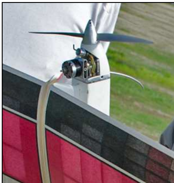
Bruce Hannah flying his replica of the Ray Monks model Beautiful workmanship revealed with OS Max 15 Max III neatly installed on very short nose
