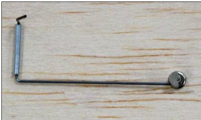
D shaped vibrator weight (facing rearward) Used to trap release arm
