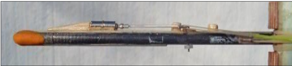
Top View shows T-Pin DT release arm engaged in Pager Motor cavity and pivot through fuselage boom with push fit Nylon keeper
