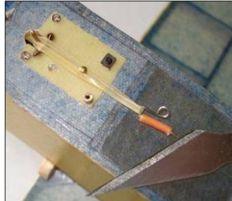
Burley Band-Burner electronic timer, available with connector for RDT release Total installation weight under 3.5gm
