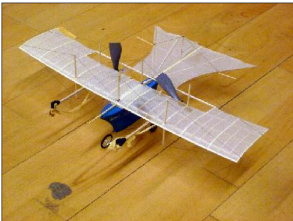
The brilliant modeller, Peter Smart, built an indoor flying model of the Aerial Steam Carriage of William Samuel Henson and John Stringfellow, which was patented in 1842. As can be seen, it has twin rubber power motors and was probably entered in Open Rubber
