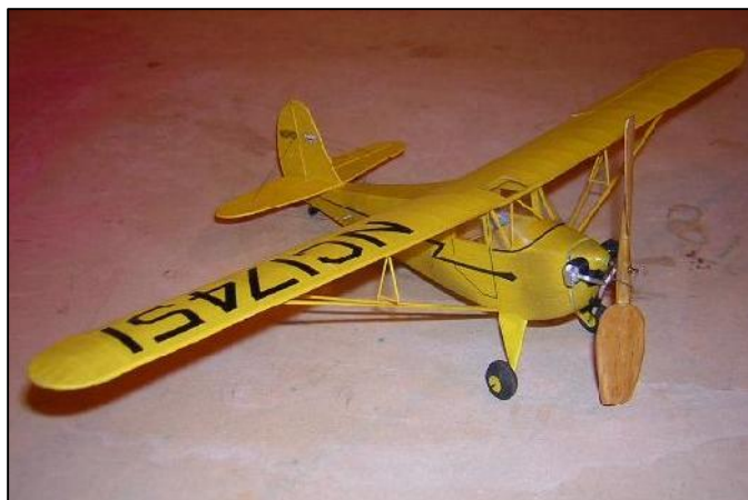
Aeronca K. 9" fuselage length Peanut 8.3g without rubber
