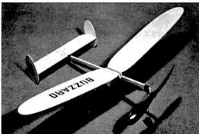
The twin-finned BUZZARD is capable of taking off under its own power from the ground. The detachable wing is held on with rubber bands.
