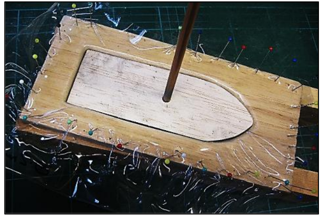
Forming the Thunderbolt canopy. The plastic is simply held in place by pins.
