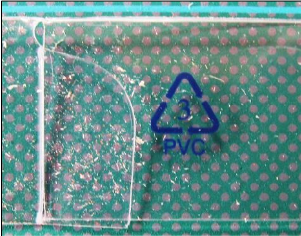
Printed chasing arrow symbol for PVC from transparent box lid. This material was used for the Zero canopy
