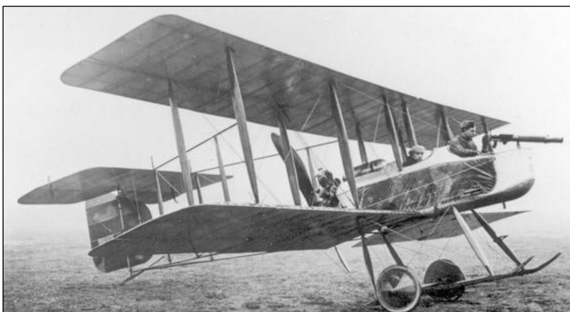
The production version of the Vickers Gunbus, showing its flexible machine gun mount in the nose. Photo: Wikipedia.
