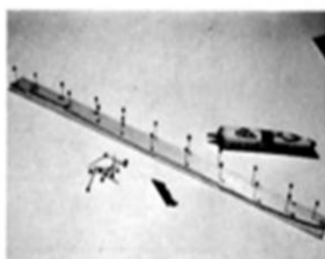
Pin fuselage core (A) over one of 'B' sides. Add other side later.
