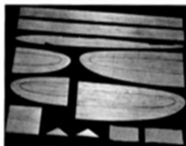
Shaped parts for SWALLOW. Note the trimming lines on flying surfaces.
