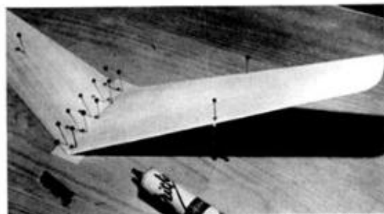
Join wing panels together at correct angle by packing up with piece 'Z'. Hold in place with pins until dry.
