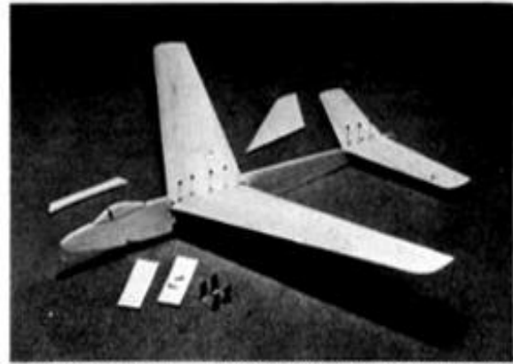
Cement flying surfaces to the fuselage, allow to dry, then replace piece of sheet over wing and add the fin.
