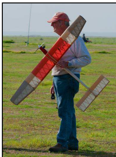
Dr. Stan Hill VTO's an earlier development version of Amazoom, note straight rib layout. Streamlined engine, tank and timer installation mostly concealed inside fuselage, note mini-Comp Screw !
