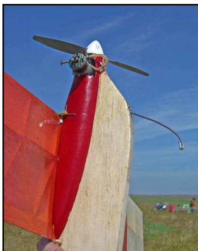
Dr. Stan Hill VTO's an earlier development version of Amazoom, note straight rib layout. Streamlined engine, tank and timer installation mostly concealed inside fuselage, note mini-Comp Screw !
