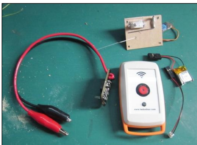
Stand Alone system with nano servo and rat-trap dt release on mounting plate.
