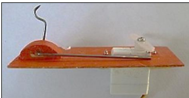
The simple 'mousetrap' system on a plate – very little force is placed on the servo.
