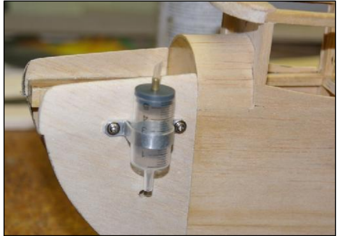
Fuel tank made from 10cc syringe in location.
