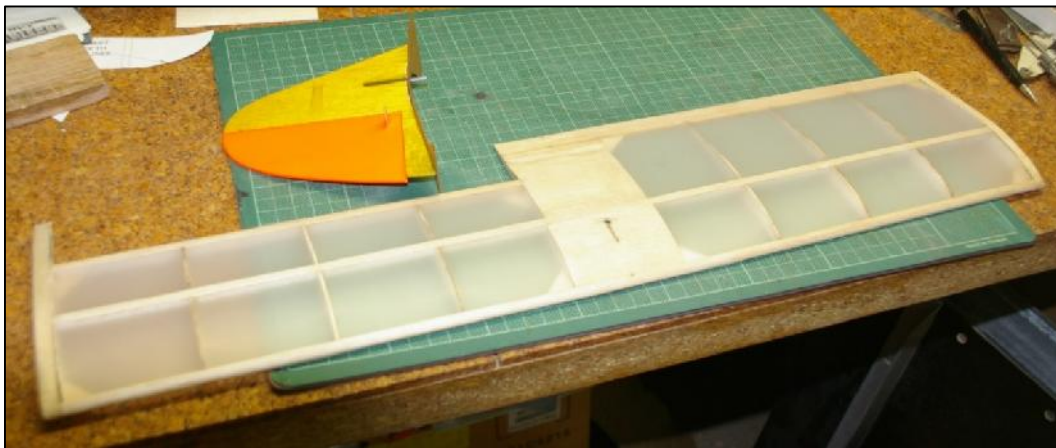
Tailplane and rudder showing locating system, carbon rod in rudder aluminium tube in tailplane with milliply rudder support and elastic band holder.
