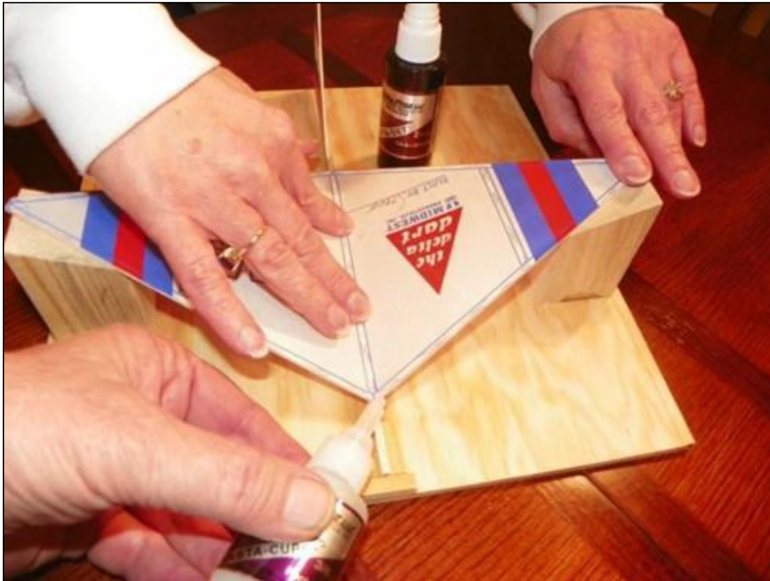
The Delta Dart Assembly Jig
