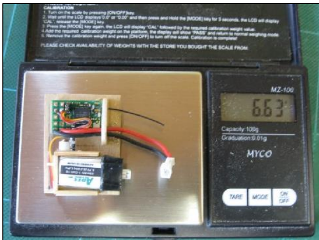
RDT components mounted on 0.8mm ply board. The battery tray is mounted on the servo.
