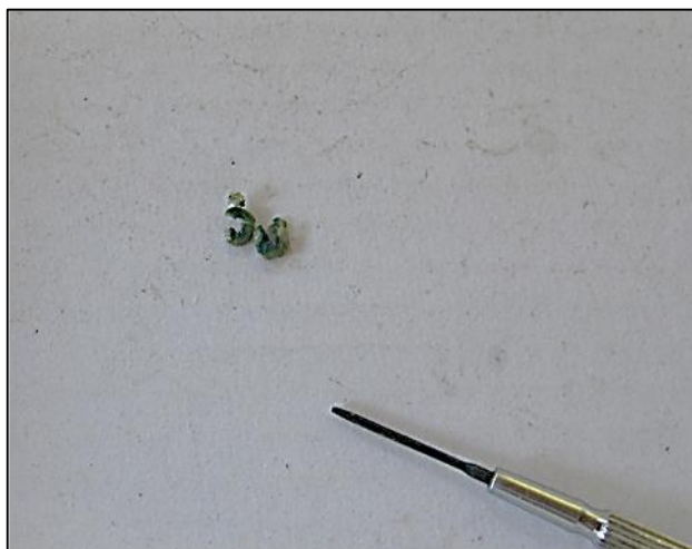
Fig 1. CO 2 motor problems - the failed seal between the copper pipe and the gland nut to the cylinder head of a Campus A-23.
