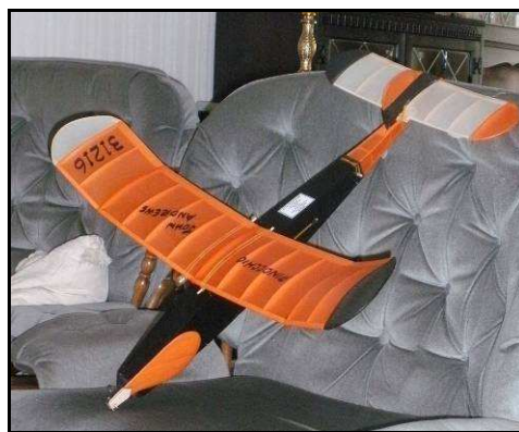
The model, somewhat fatter at the nose for the winding tube, and bamboo tips cos I can't bend balsa
