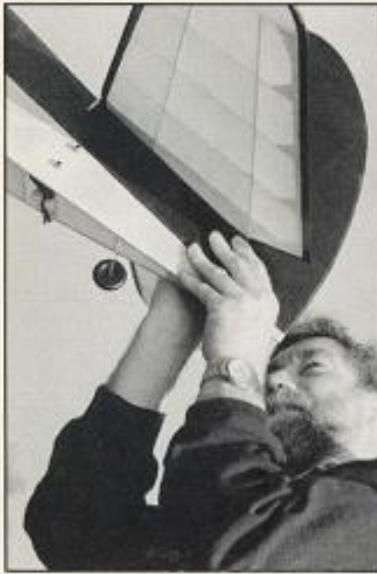
The tailplane is secured by the fin, an arrangement that did not allow sufficient adjustment. Easy to alter but not on the field.
