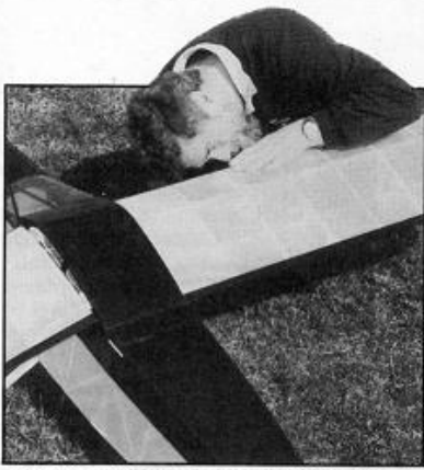
Model assembles easily; break in the two-piece fuselage can just be seen behind wing where it is held by a small rubber band at each corner.
