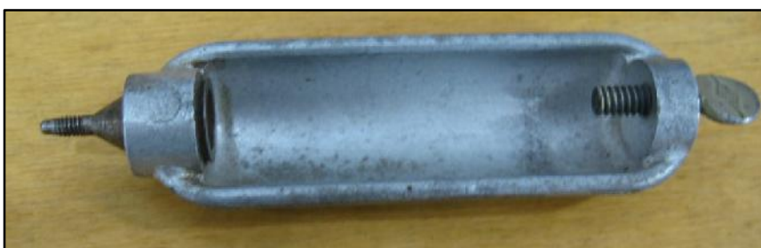
Original Brown holder for CO 2 capsule with screw-in tank connector for late 1940s Campus motors. Replica tank filler valve, made by Gerard Moore alongside.
