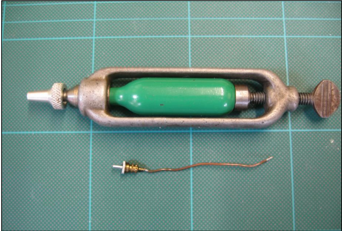
!970s holder for CO 2 capsule, with ball valve, for Brown '005' and later motors. Remote tank filler valve below
