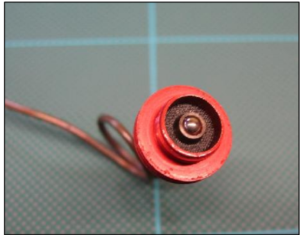
Cylinder head of conversion showing ball valve
