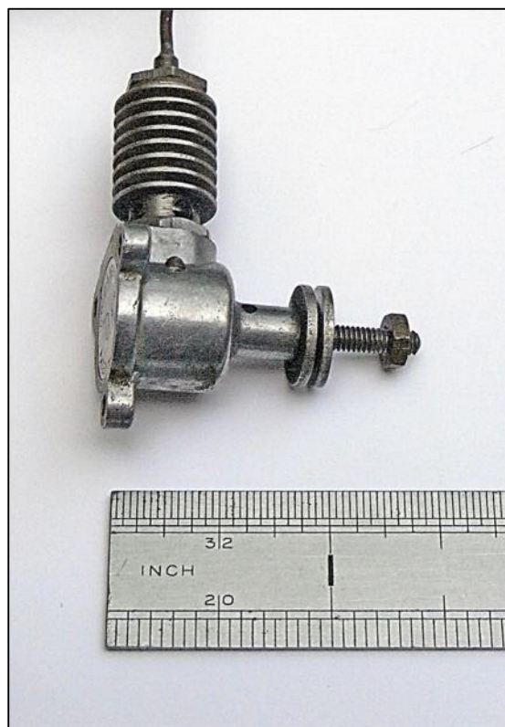
Close-up of OK motor. The lubrication holes are clearly visible.
