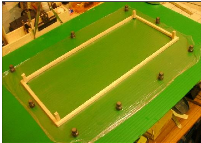
Vaseline coated 3/8 sq framework dropped on film
