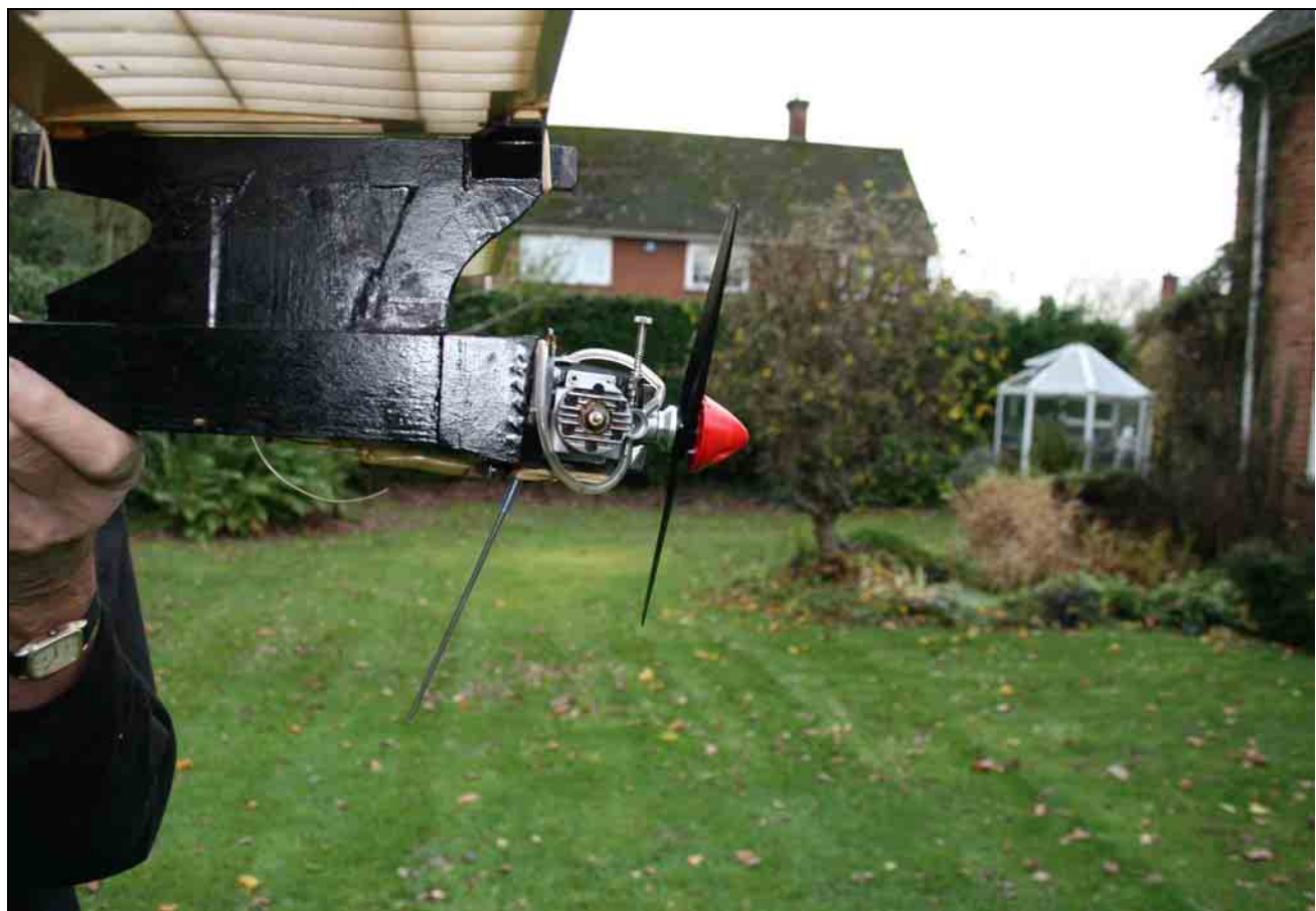
Mr Max, showing engine downthrust
