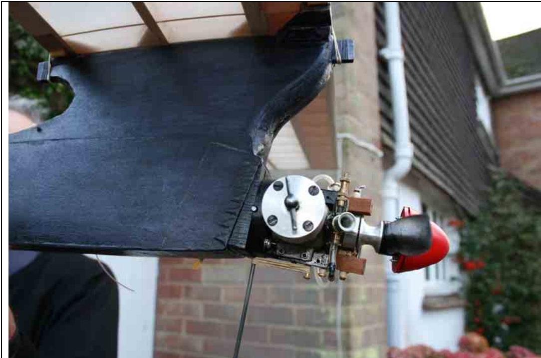
Downthrust angle on Ranta's design
