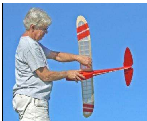
Bill assembles the model and then fits the 1/8 th incidence packing
