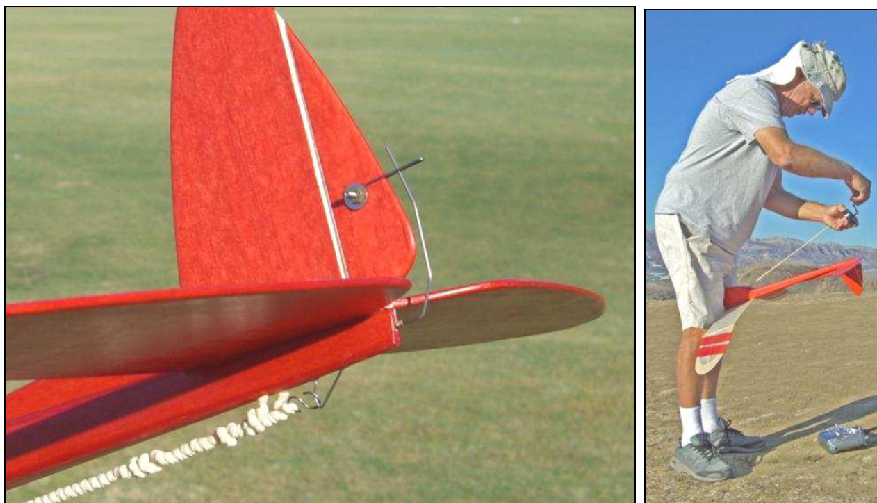
Tail surfaces showing torque rod for rudder & rubber motor for actuator power, needs winding occasionally.
