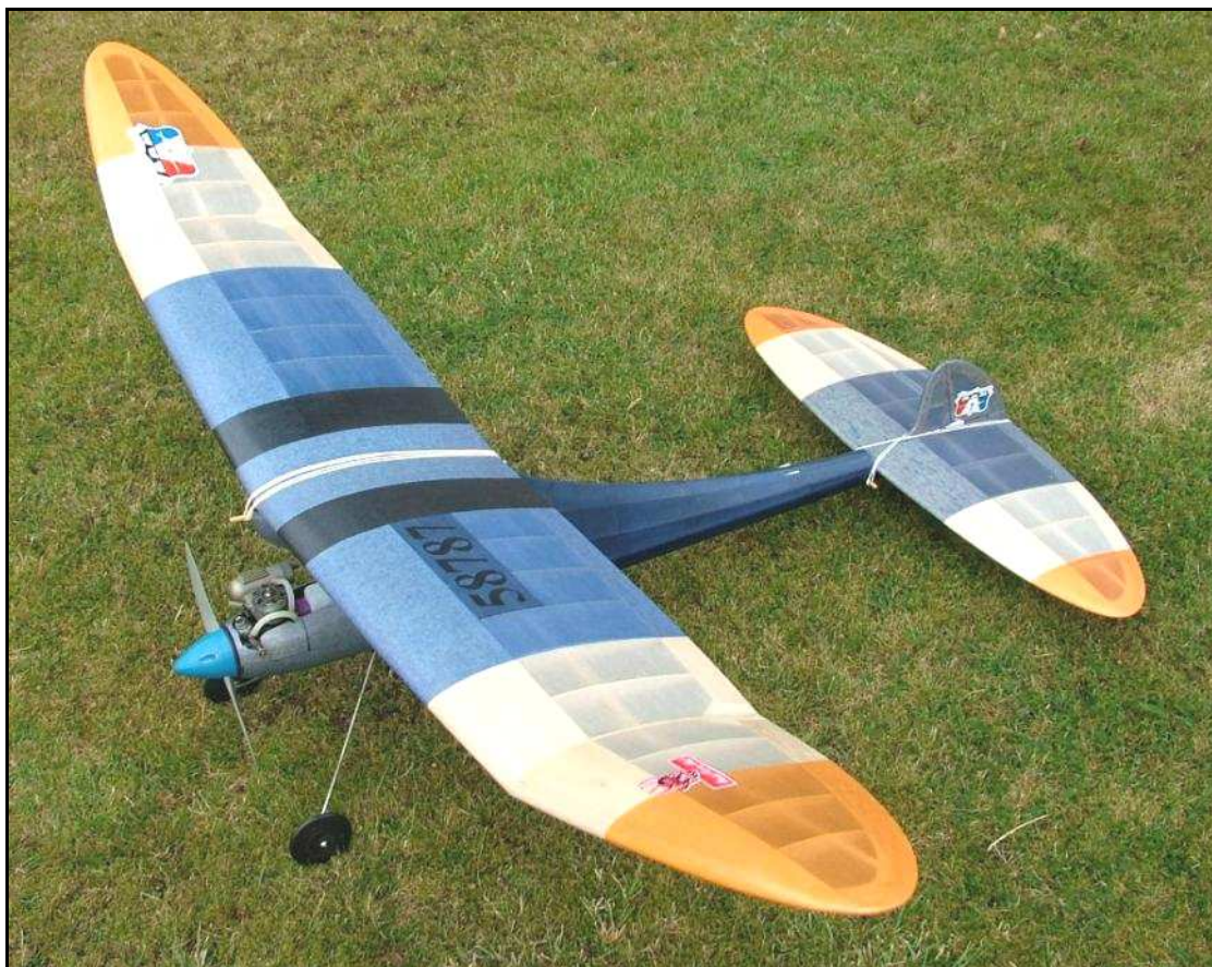
An R/C 'Super Slicker' by Colin Shepherd 3 function radio, one on engine, originally OS25 powered but now with OS20 (Colin thought it was a bit too lively with the 25)
