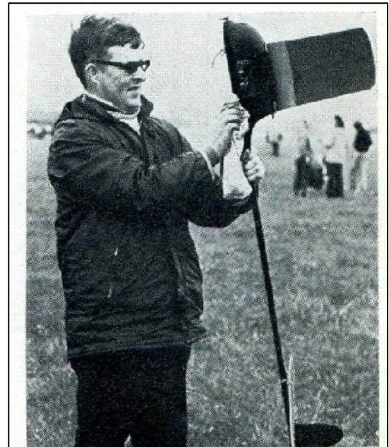
Tom Smith used new F.A.I. design 'Noggin'. All-sheet surfaces employed. Rossi 15 hides inside glassfibre cowl-cum-pylon blended into Ronitube boom.
