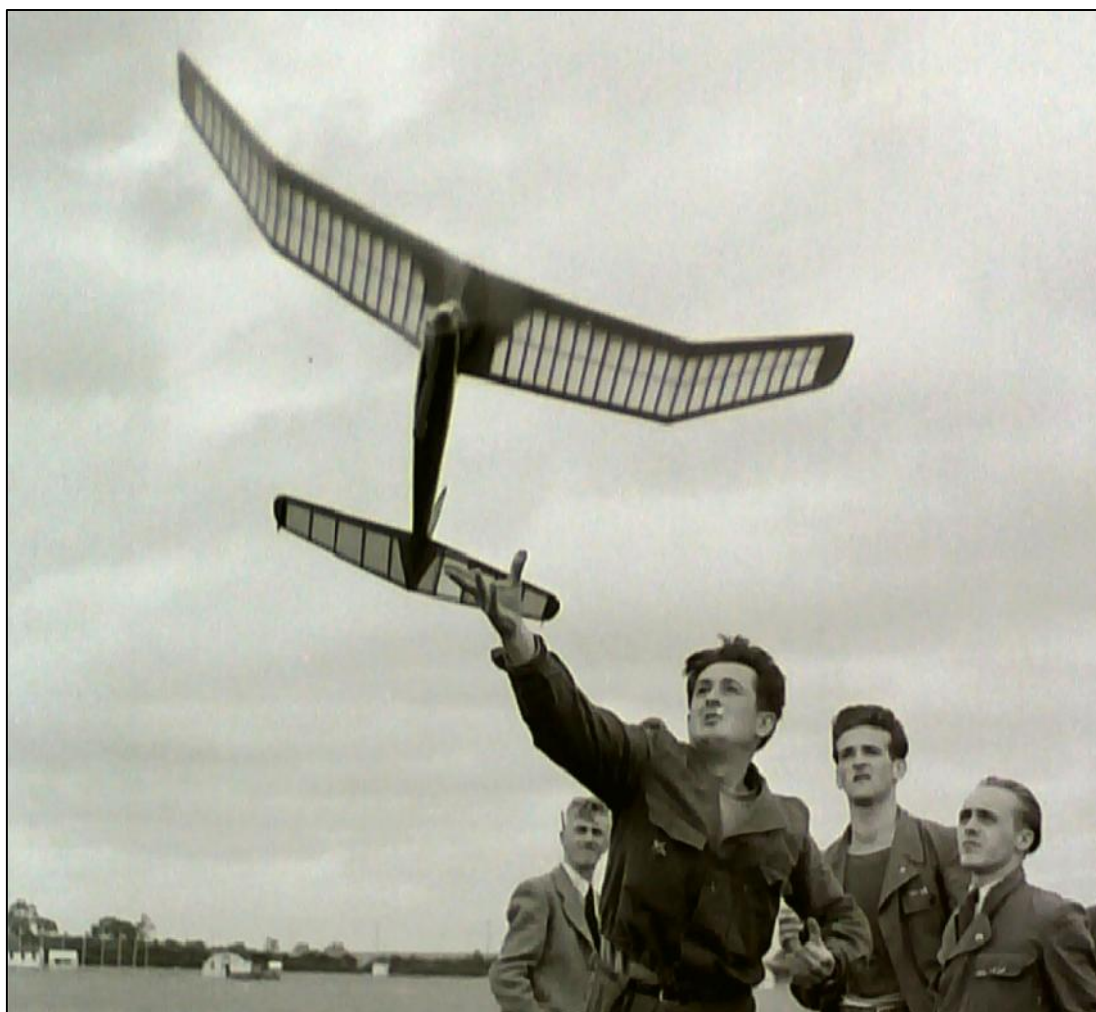
Draga Zigic of Yugoslavia, assisted by Zdenka Juresa, launches his "W" power model at the 1950 Eaton Bray International meeting. Model features folding prop and retractable undercart. Photo used as frontispiece in the December 1950 Aeromodeller.
