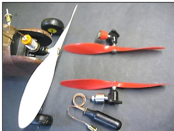
Three motors with the same moulded crankcase. From the left, clockwise: - Tornado 69, Shark without pipe-work, Mistral.
