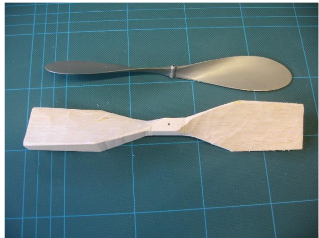
Fig.3. Rear view of balsa prop with carved blade form.
