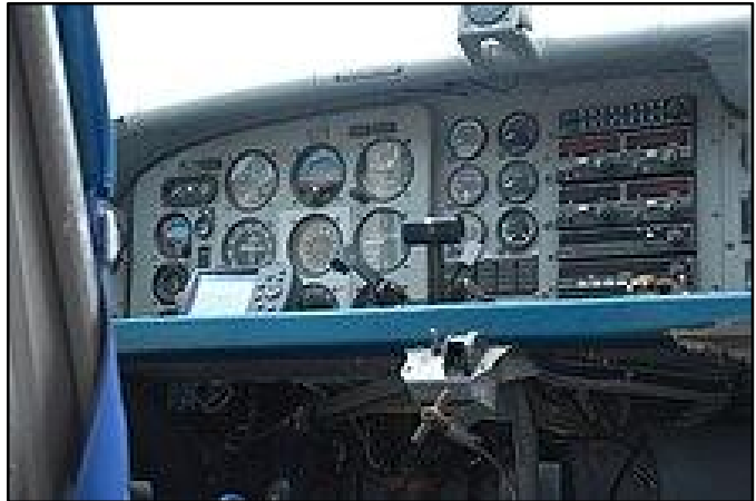
Analog cockpit instrumentation of a PC-6, 2007
