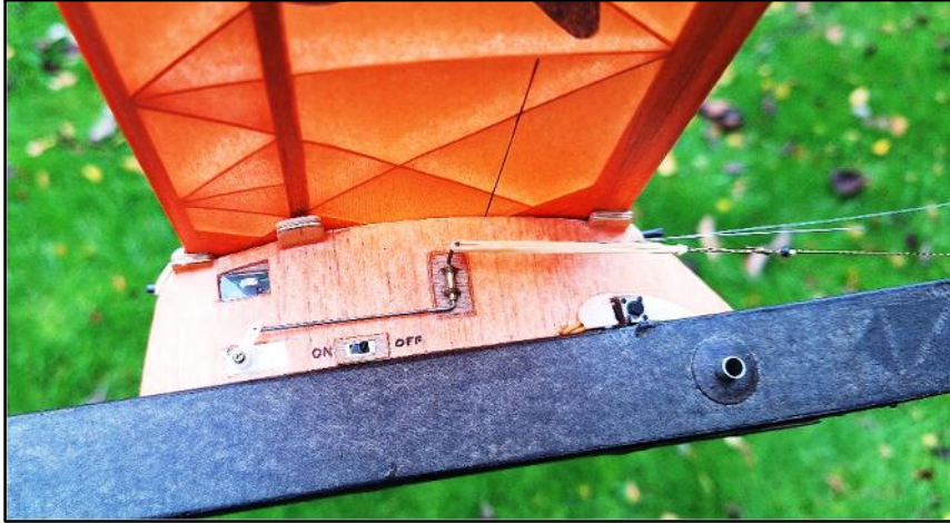
Pylon on finished model showing servo D/T release, on/off switch, push button start switch and window to view the e-timer bright-blue LED.
